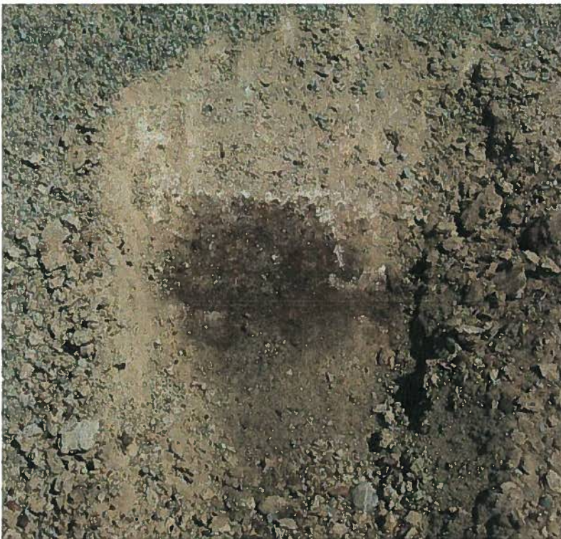
Figure 15. SA 4. Soil profile buried beneath approximately 8 inches of serpentine sediment. The buried, well-developed Henneke soil series has a dark A horizon enriched in organic matter.
